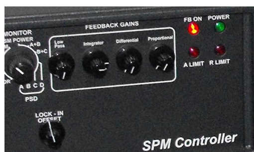
Figure 56: FB ON Indicator on SPM Controller
