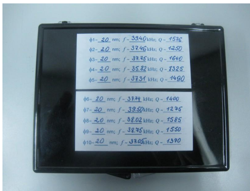
Figure 12: Tip-mount Box - Back View, with Tip Parameters
