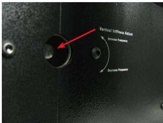
Figure 84: Vertical Stiffness Adjustment
