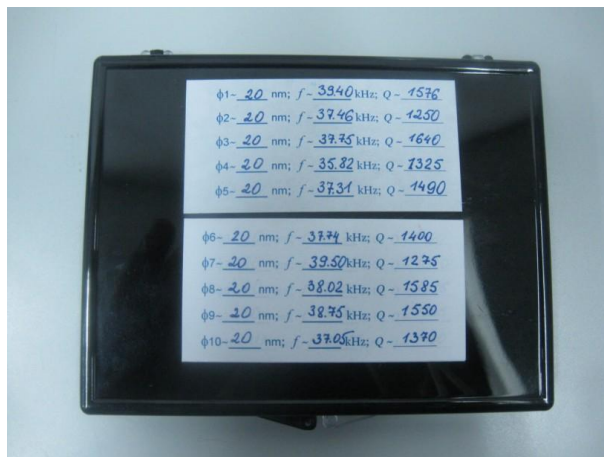
Figure 33: Back of AFM tipmount case, showing tip parameters
