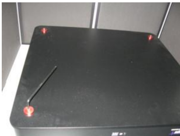
Figure 76: Releasing Plate Screws
