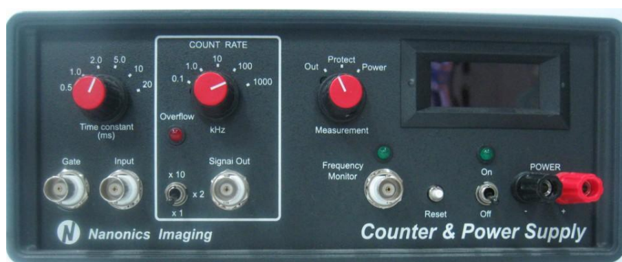
Figure 25: APD Counter and Power Supply
