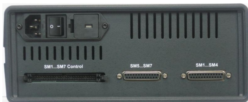
Figure 24: Multi-channel Stepper Motor Driver – Rear Panel
