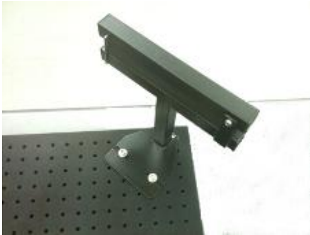
Figure 82: Cable Management System
